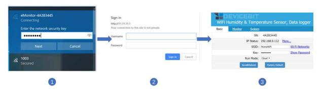
**Step1**, Use your smart device's Wi-Fi connection setup, connect to the Monitor's network, which will show up as eMonitor\_xxxxxxxxx (xxxxxxxxx is unique device SN). No password required.
